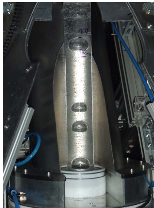
Figure 3. Snapshot of the in-house developed ultrafast electron beam X-ray tomography along with slug flow at U_G = 0.034 m/s and \mu_L = 1149 mPa-s (100% glycerol).
